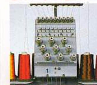
▲ UNDER THREAD DETECTOR (UTSM) Embroidery machine automatically stops when under thread gets cut or runs out.
